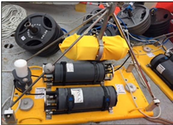
Figure 4-9. Recorder configuration on bottom plates with hydrophones mounted ~0.5m above the seabed. The upper cylinder is the recorder, the lower cylinder is a 48-D-cell alkaline battery pack.
