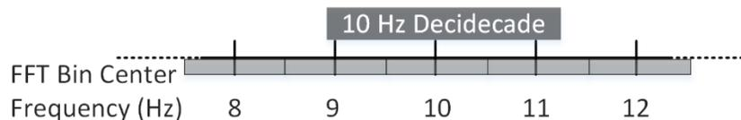
Figure 2-6. Overlap of the 10 Hz decidecade frequency band on a 1 Hz resolution frequency axis.
