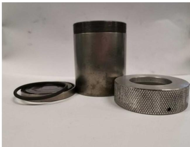
Figure 3.1 The different parts of a SPEX milling vial.
