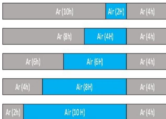
Figure 3.2 Scheme of ball milling procedures for different  $\text{Si}_{85}\text{Fe}_{15}\text{O}_x$  alloys.
