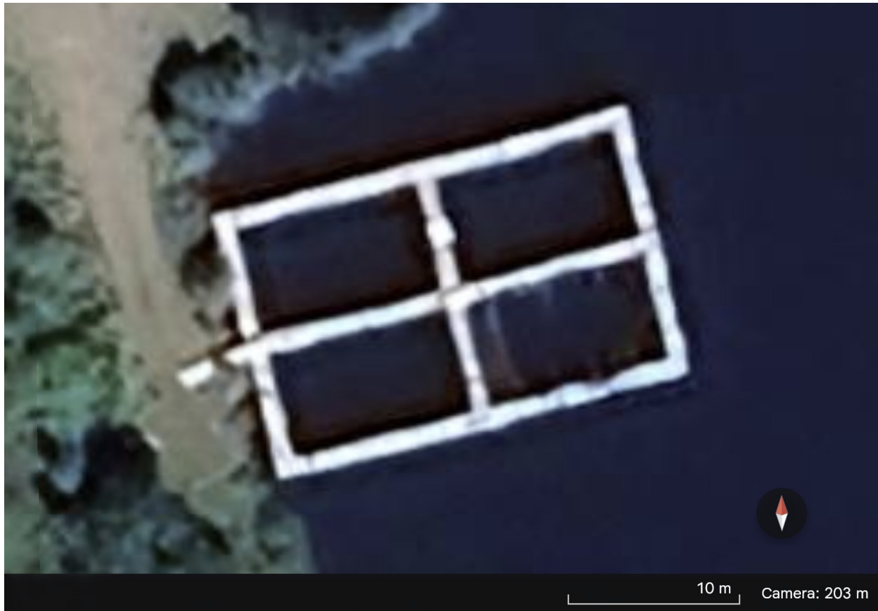
Figure 3.1. Aerial photo of North River Fish Farms Ltd.'s Middle Pond, with its four visible rearing cages (6.1 x 12.2 x 3.7 m. deep). Altitude of 203 m. Source: Google Earth, 7 June, 2025.
