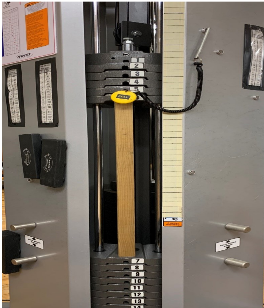
Figure G.3: The leg press weight plates being lifted up with the help of wooden plank support.
