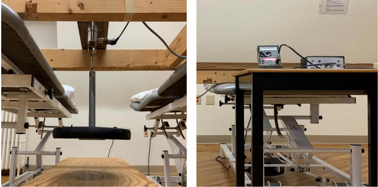
Figure G.1: Free weight supported by the weight pan suspended from a load cell. (left) The load cell is connected to an amplifier and multimeter (right).
