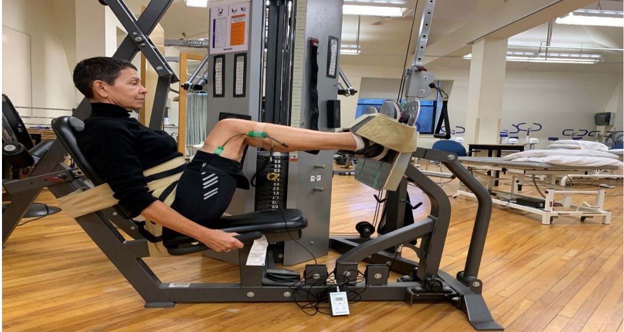
Figure 1: Participant seated on the leg press seat with an electronic goniometer attached, feet placed on the markings, waist-hip-feet stabilized with the belts.
