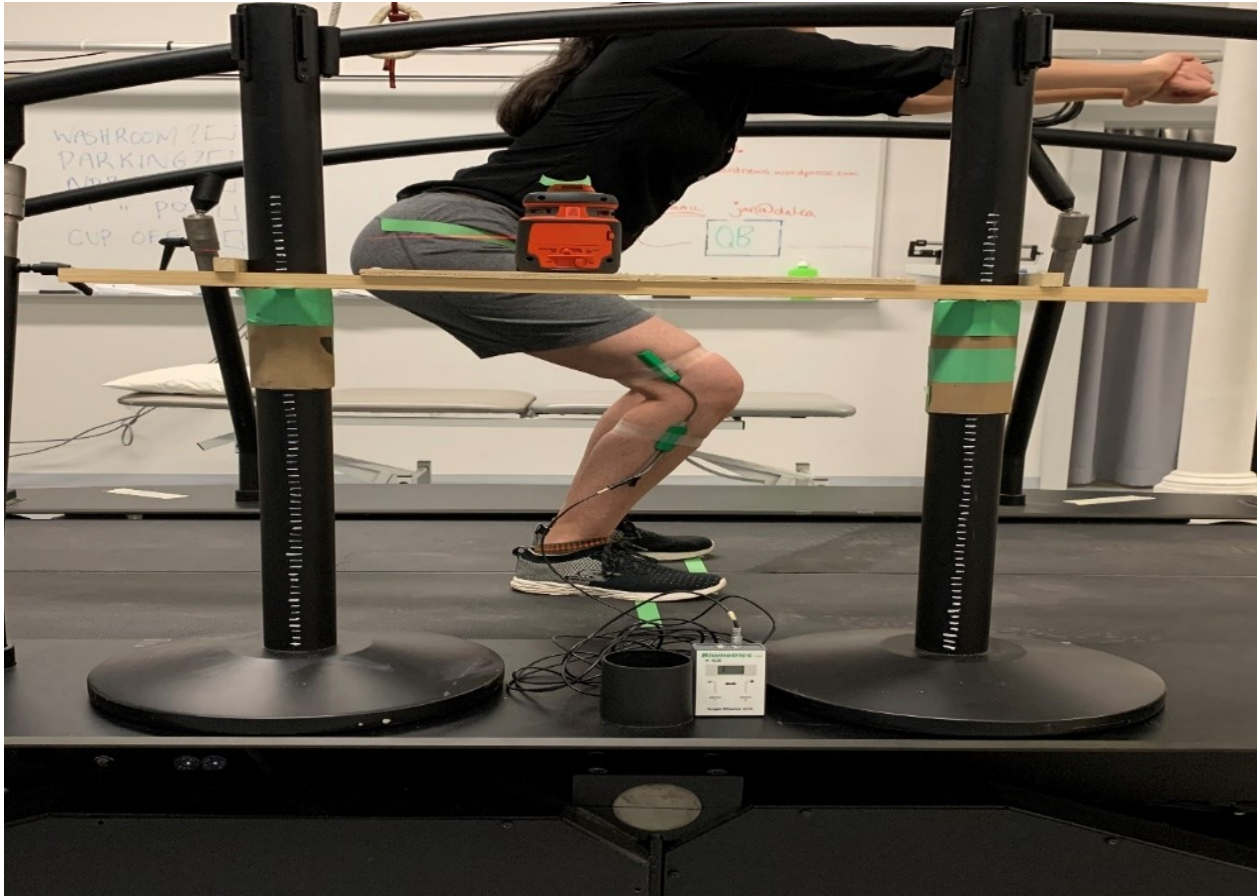
Figure 4: Participant performing a squat on the force plate with electronic goniometer recording the right knee angle and squat height matched with the laser light.
