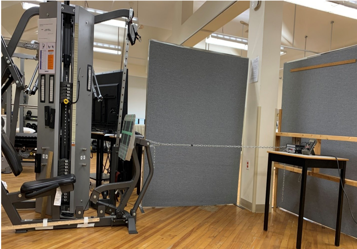
Figure G.2: The leg press configuration to assess the accuracy of the Hoist weight plates. The metal chain connects the leg press foot plate and the load cell. The load cell is connected to the voltmeter via the amplifier.
