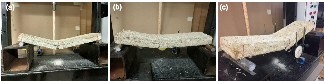
Figure 3: Failure modes: (a) Beam 1; (b) Beam 2; and (c) Beam 3
