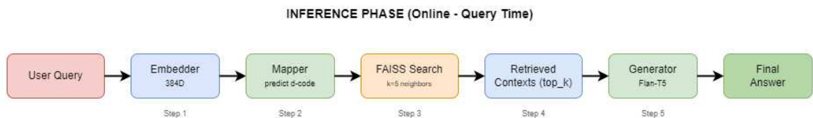
Figure 3.1: Inference phase: Complete query processing pipeline. User query is embedded with Sentence-BERT producing 384D representation (Step 1). Trained mapper predicts d -dimensional compressed code via single forward pass (Step 2). FAISS searches pre-built compressed index for k = 5 nearest neighbors in compressed space (Step 3). Corresponding context texts are retrieved from database (Step 4). Retrieved contexts provide information for Flan-T5 to generate final response (Step 5). All retrieval operations occur in compressed d -dimensional space.
