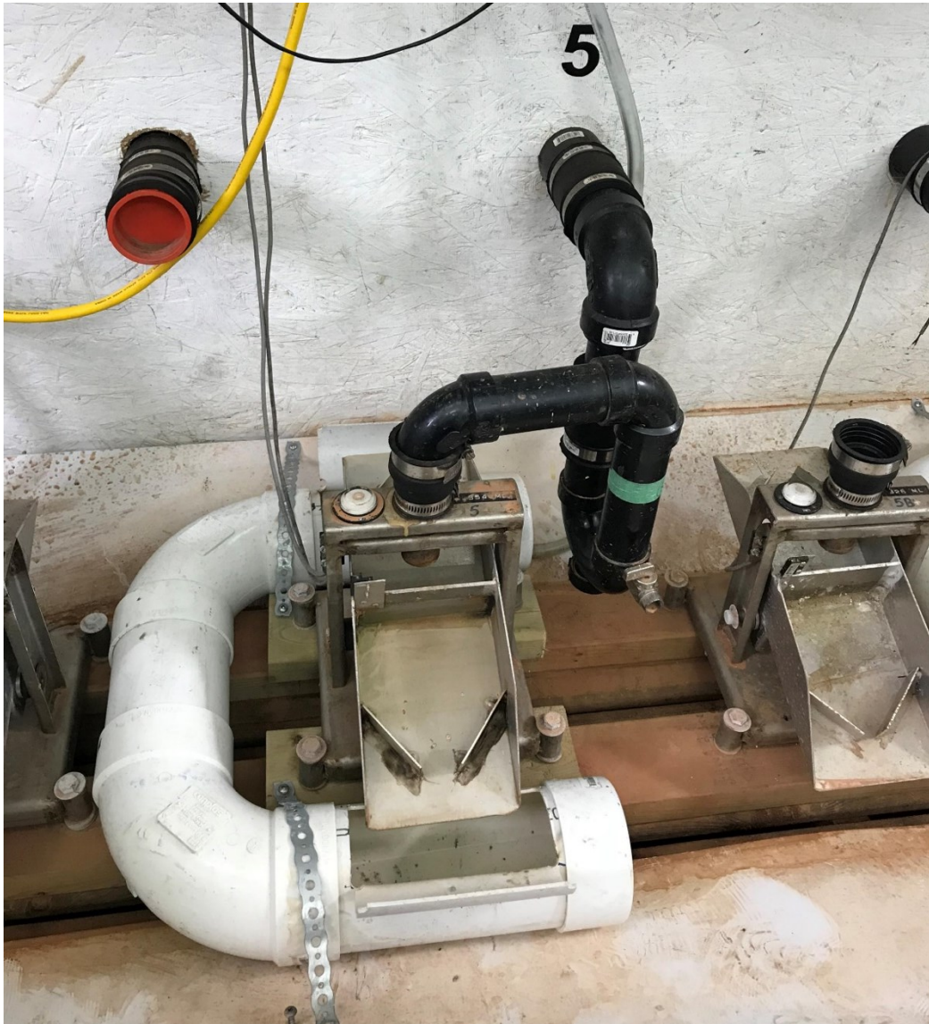
Figure C.3. Picture of drainage and calibrated tipping bucket set up connected to the lysimeter cell 5.
