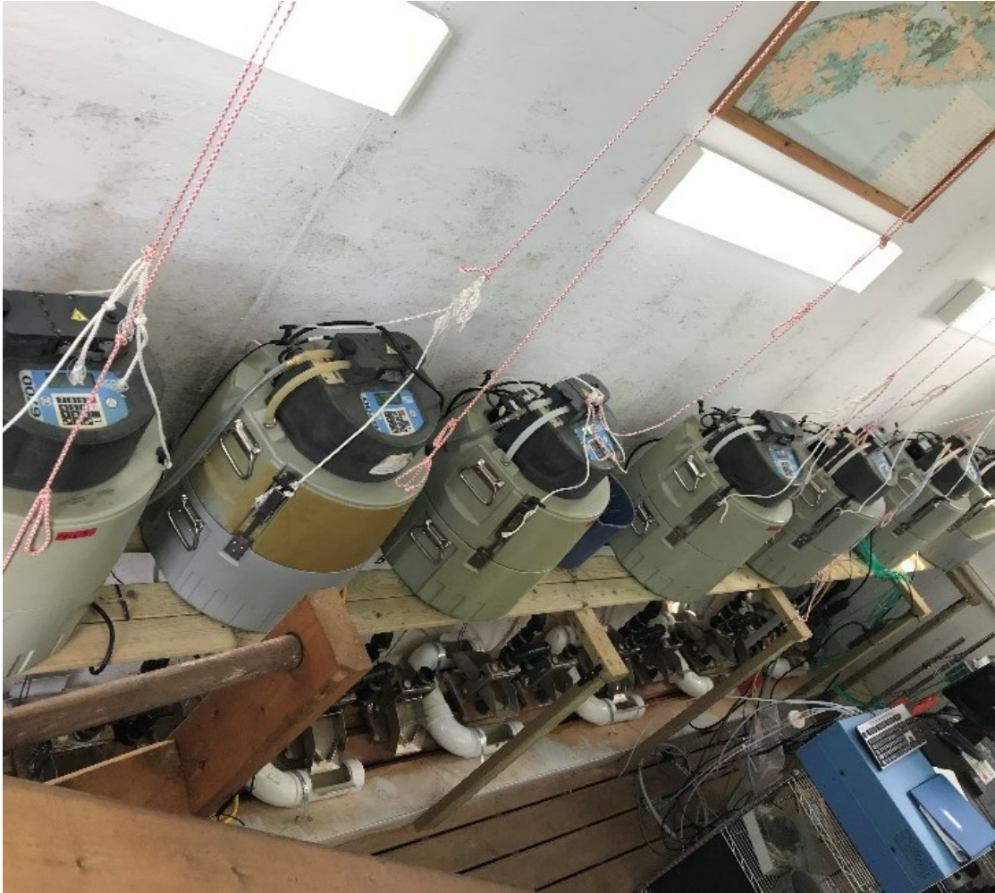
Figure C.2. Picture of ISCO 6700 Full-size Portable Sampler (Teledyne Isco, Lincoln, NE, USA) set up for the lysimeter cell study.
