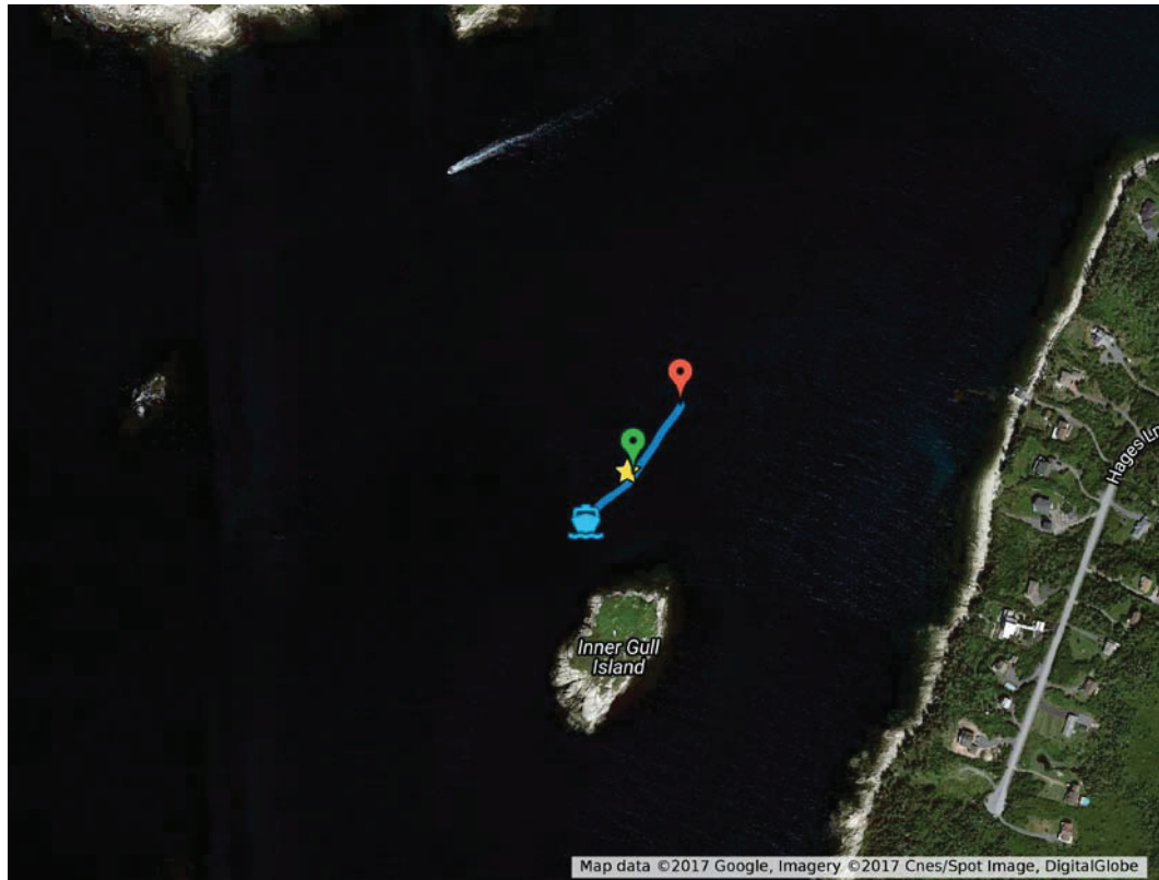
Figure 5.4: Demonstration of the location of the sea trial on the map. The total traveled distance is 161m. The maximum measured speed is 0.9 \frac{\text{m}}{\text{s}} . The boat icon shows the point that the boat started drifting. The star shows the location of the transmitter. The green icon represents the point where the receiver started recording and the red icon shows the point where the receiver stopped recording.
