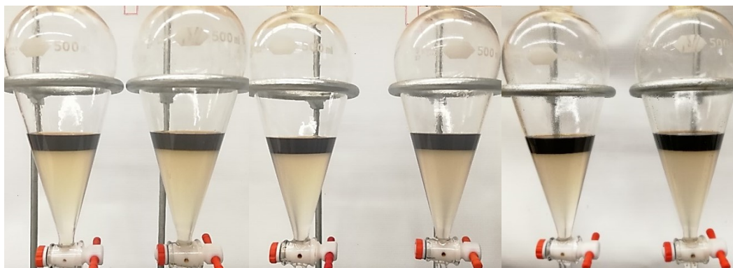
Figure S.11 Phenomena observed in funnels containing “A”, “N”, and “B” filtrates from alkaline lignin when emulsions were broken
