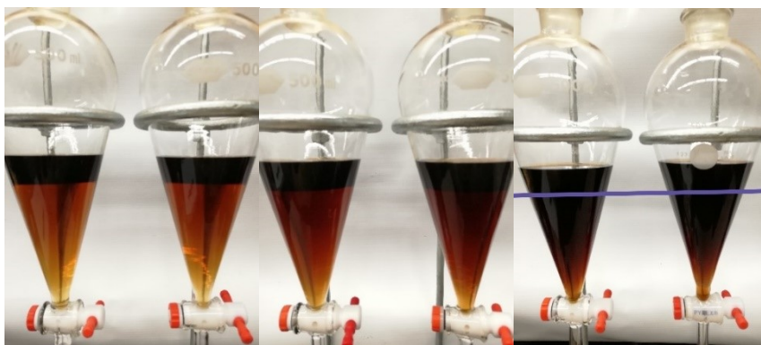
Figure S.4 Phenomena observed in funnels containing “A”, “N”, and “B” filtrates from de-alkaline lignin when 50ml ethyl acetate and 60ml water were added
