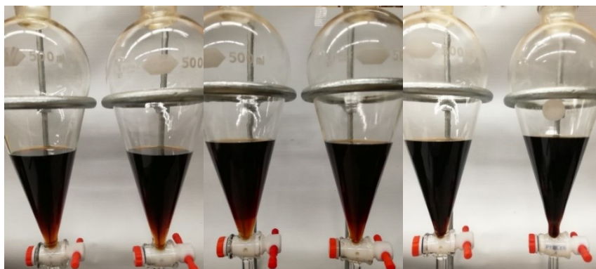
Figure S.2 Phenomena observed in funnels containing “A”, “N”, and “B” filtrates from dealkaline lignin when 50ml ethyl acetate was added
