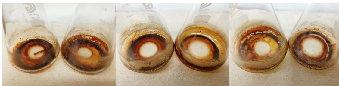
Figure S.14 De-alkaline lignin BO derived from “A”, “N”, and “B” filtrate
