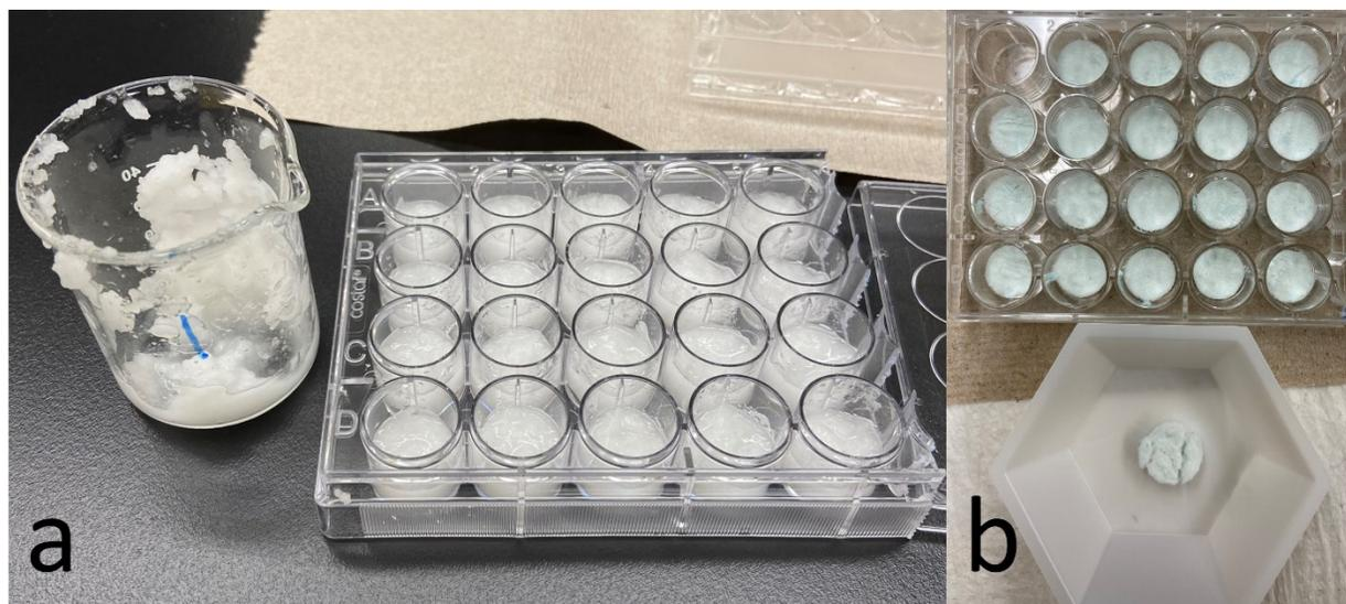
Figure 5 – The paste-like gel polyelectrolyte complex made using the homogenizer (a) and the resulting freeze-dried material (b).
