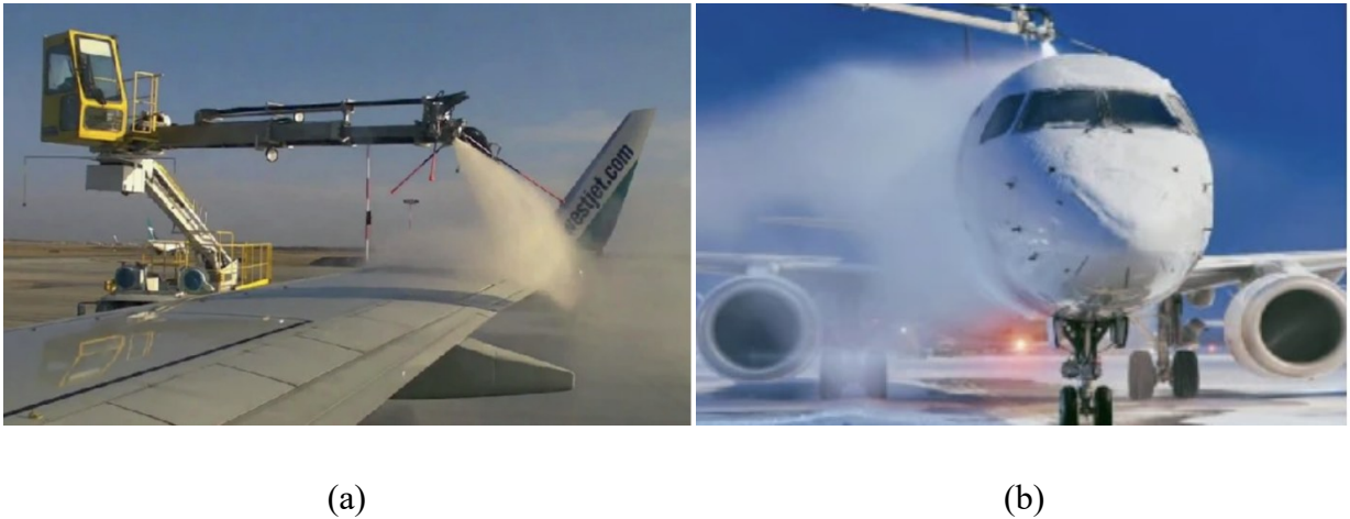
Figure 2.2. Diagram showing (a) spraying of high temperature chemicals on aircraft wing before takeoff and (b) spraying of high temperature chemicals on an aircraft after landing (Fu et al., 2024).
