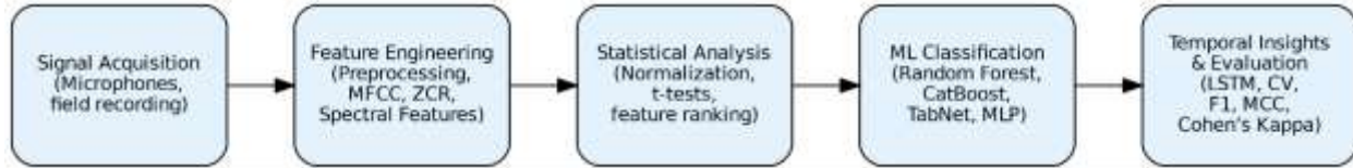
Figure 3.1 Acoustic sensing pipeline for poultry monitoring, including signal acquisition, preprocessing, feature extraction, statistical analysis, and machine learning-based classification of health, behavior, and stress states.
