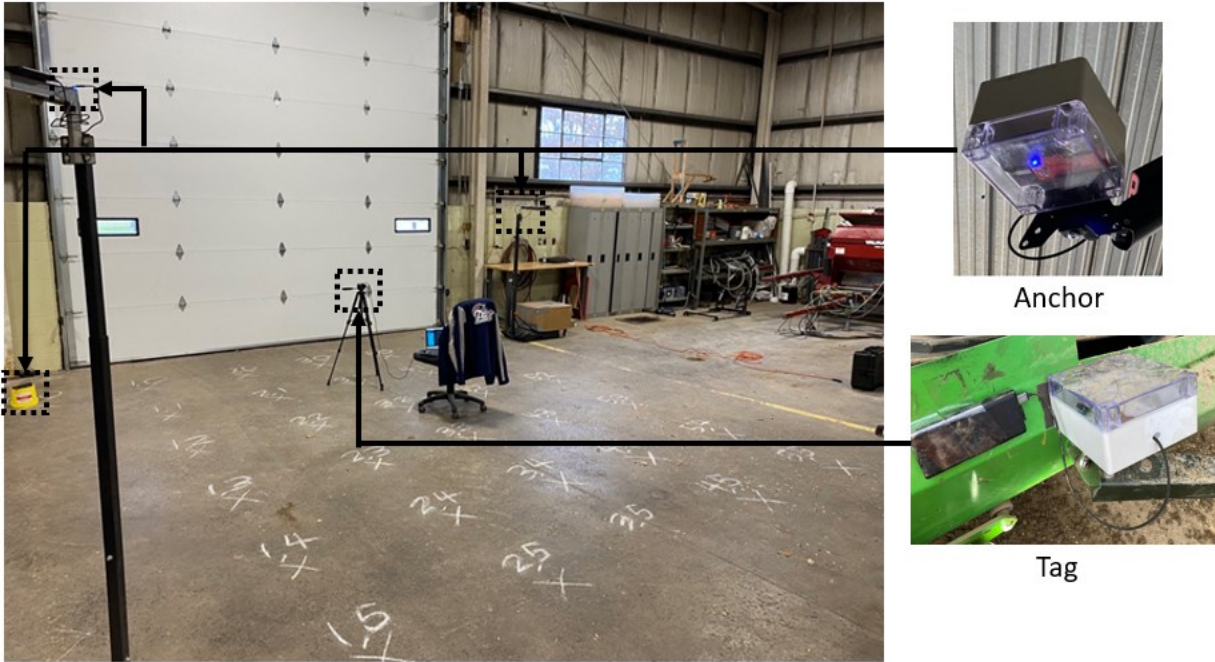
Figure 3.4: Experiment 1 Setup - Picture of obstacle-free area in lab. The tag was mounted on a tripod, aligned with each designated (X, Y) coordinate on the grid to ensure accurate determination of its actual position.
