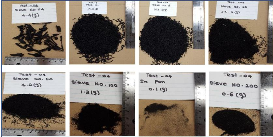
Figure 1: Various sizes shredded rubber particles used in this study
