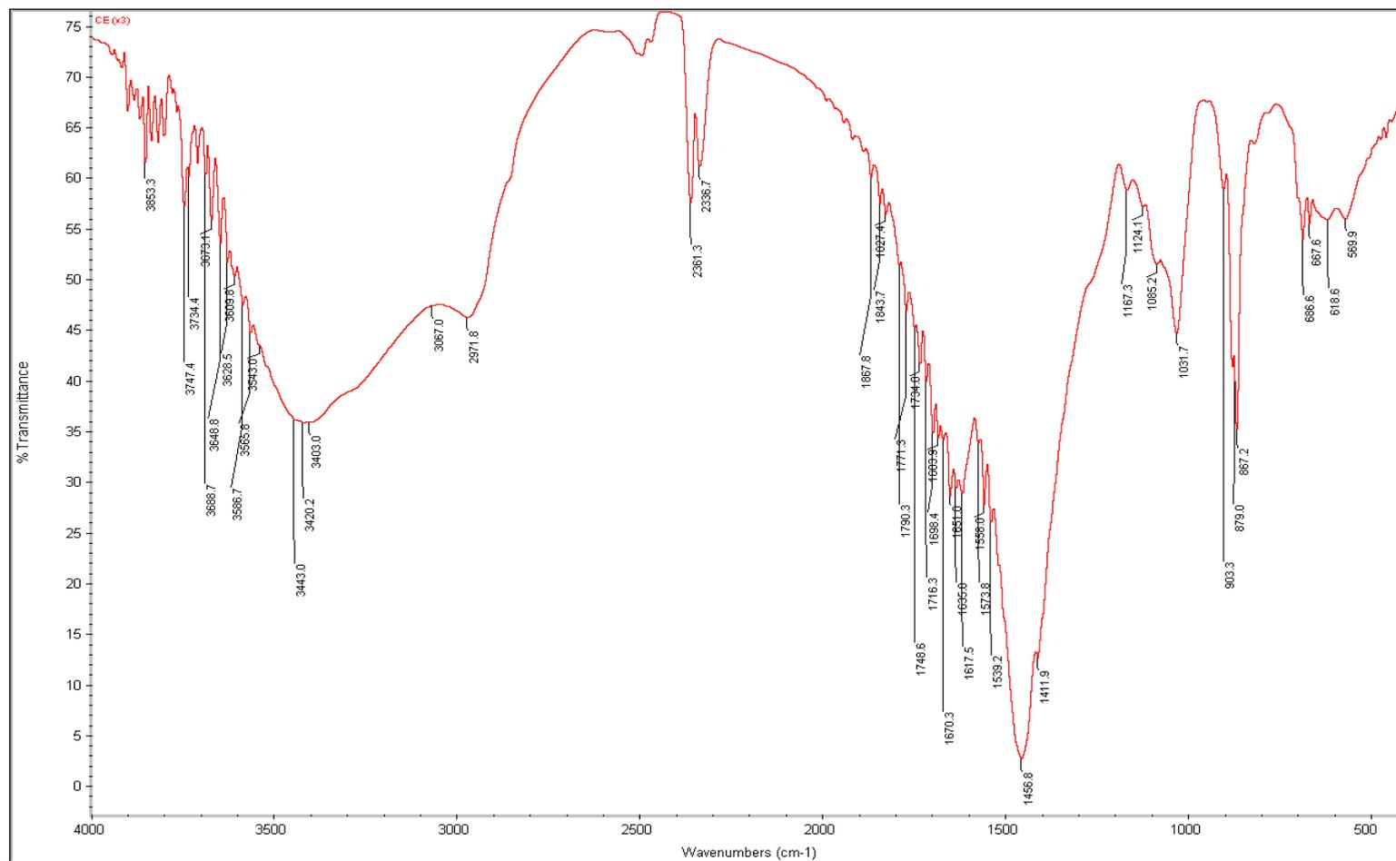
**FIG. B3. THE FTIR SPECTRUM OF SODIUM ALGINATE EXTRACT FROM CONVENTIONAL CHEMICAL EXTRACTION (Alg-CCE) (3×)**
