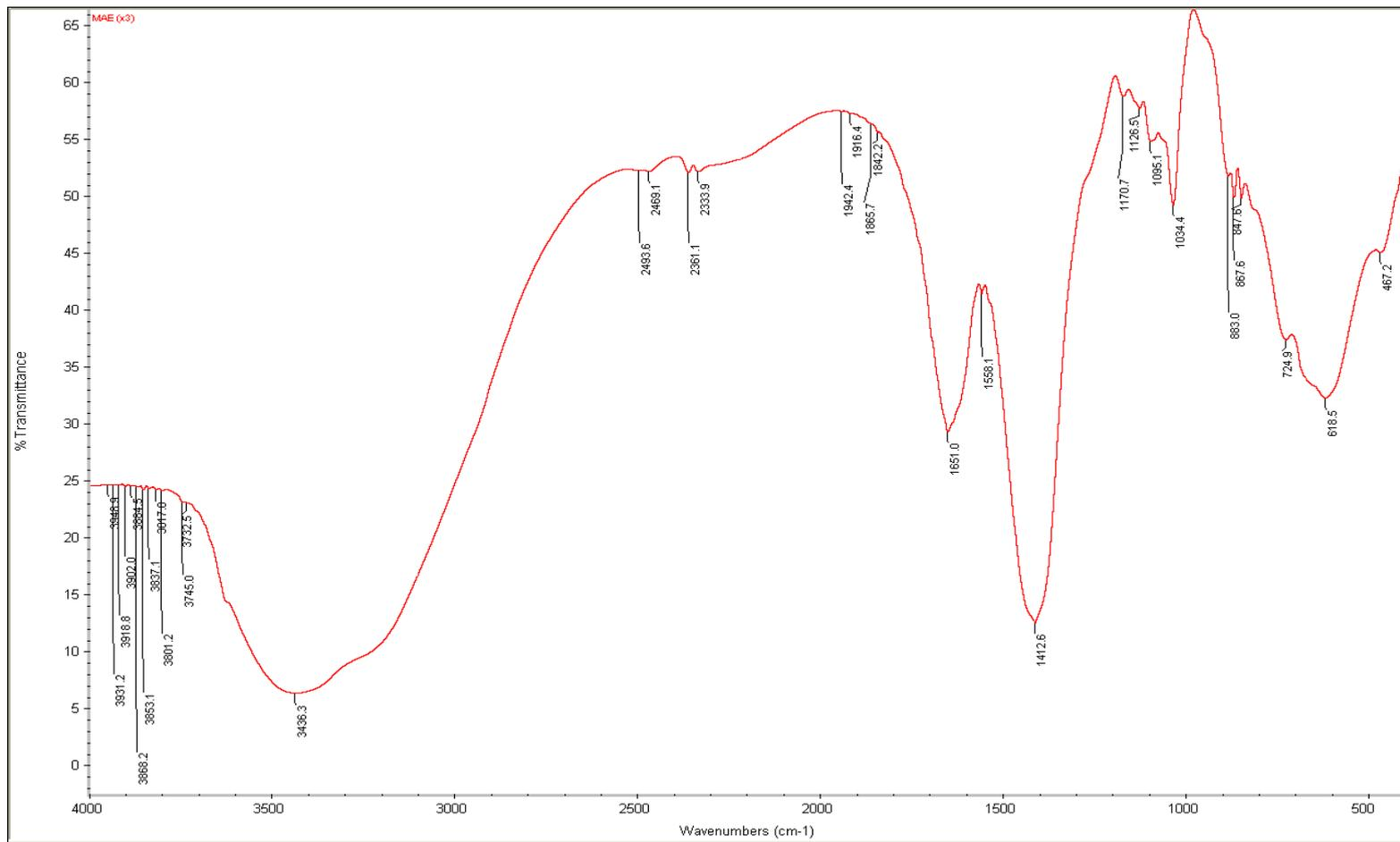
**FIG. B5. THE FT-IR SPECTRUM OF SODIUM ALGinate EXTRACT FROM MICROWAVE-ASSISTED EXTRACTION (Alg-MAE) (3×)**
