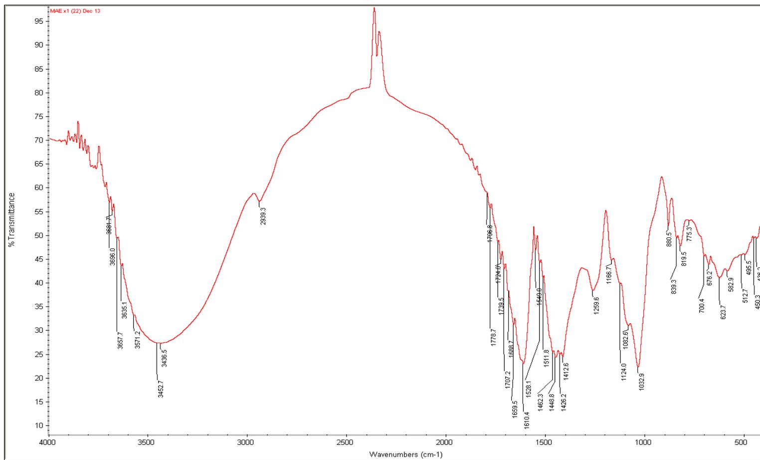
**FIG. B4. THE FTIR SPECTRUM OF SODIUM ALGinate EXTRACT FROM MICROWAVE-ASSISTED EXTRACTION (Alg-MAE) (1×)**
