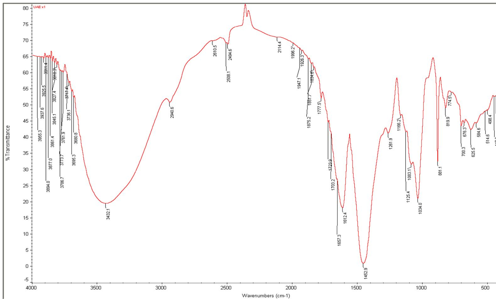
**FIG. B6. THE FT-IR SPECTRUM OF SODIUM ALGinate EXTRACT FROM ULTRASOUND-ASSISTED EXTRACTION (Alg-UAE) (1×)**
