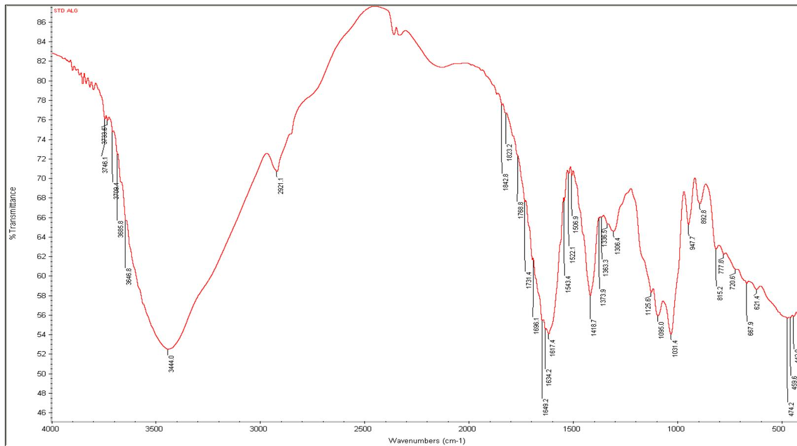
FIG B1. THE FT-IR SPECTRUM OF COMMERCIAL SODIUM ALGINATE
