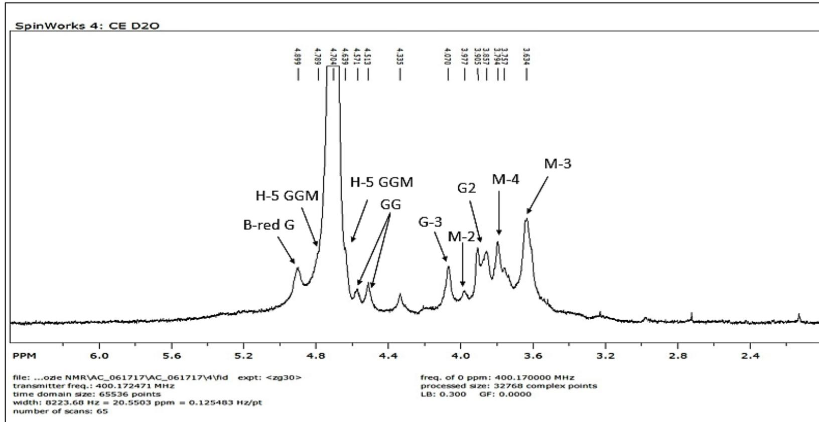
FIG 4.2. THE  $^1\text{H}$  NMR SPECTRUM OF SODIUM ALGINATE FROM CONVENTIONAL EXTRACTION (Alg-CE) ( $3\times$ )
