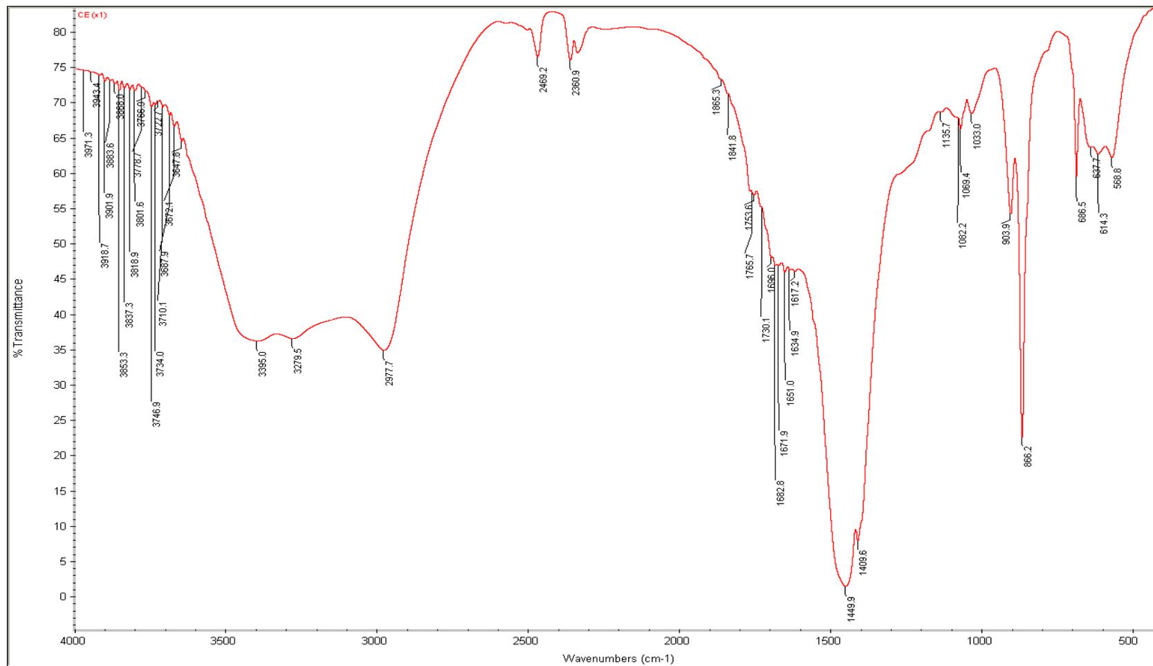
**FIG. B2. THE FTIR SPECTRUM OF SODIUM ALGinate EXTRACT FROM CONVENTIONAL CHEMICAL EXTRACTION (Alg-CCE) (1x)**
