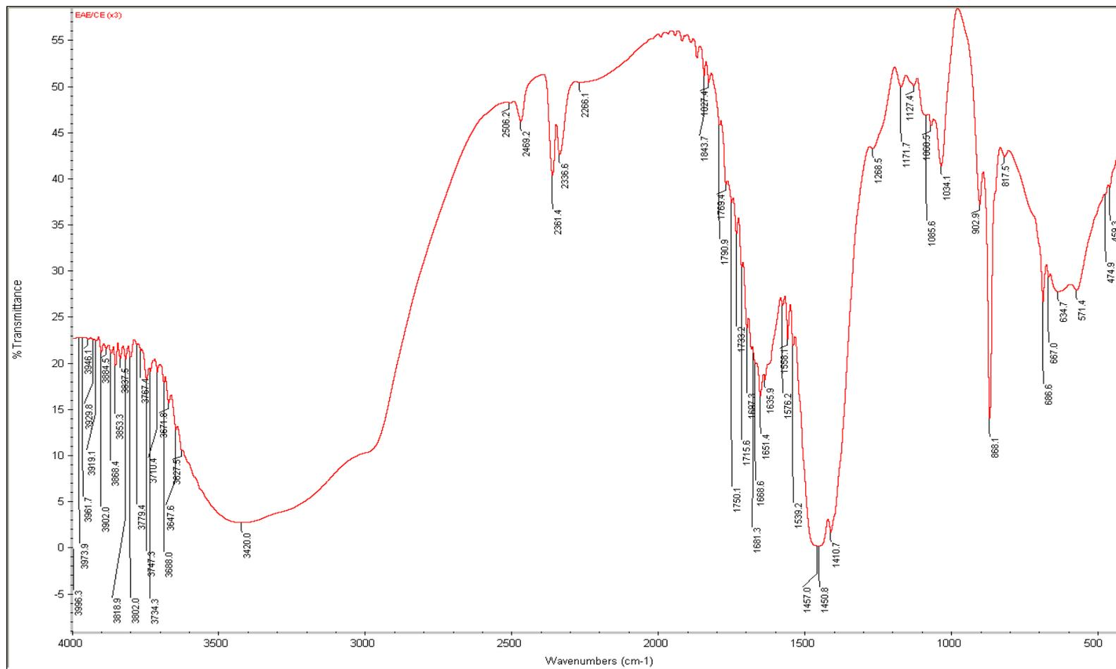
**FIG. B8. THE FT-IR SPECTRUM OF SODIUM ALGinate EXTRACTS FROM ENZYME-ASSISTED EXTRACTION (Alg-EAE) (3x)**
