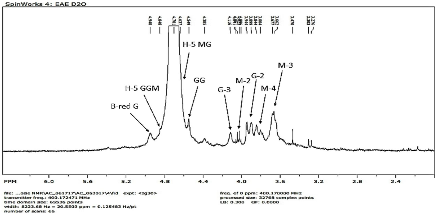
FIG 4.5. THE  $^1\text{H}$  NMR SPECTRUM OF SODIUM ALGINATE FROM ENZYME-ASSISTED EXTRACTION (3 $\times$ )
