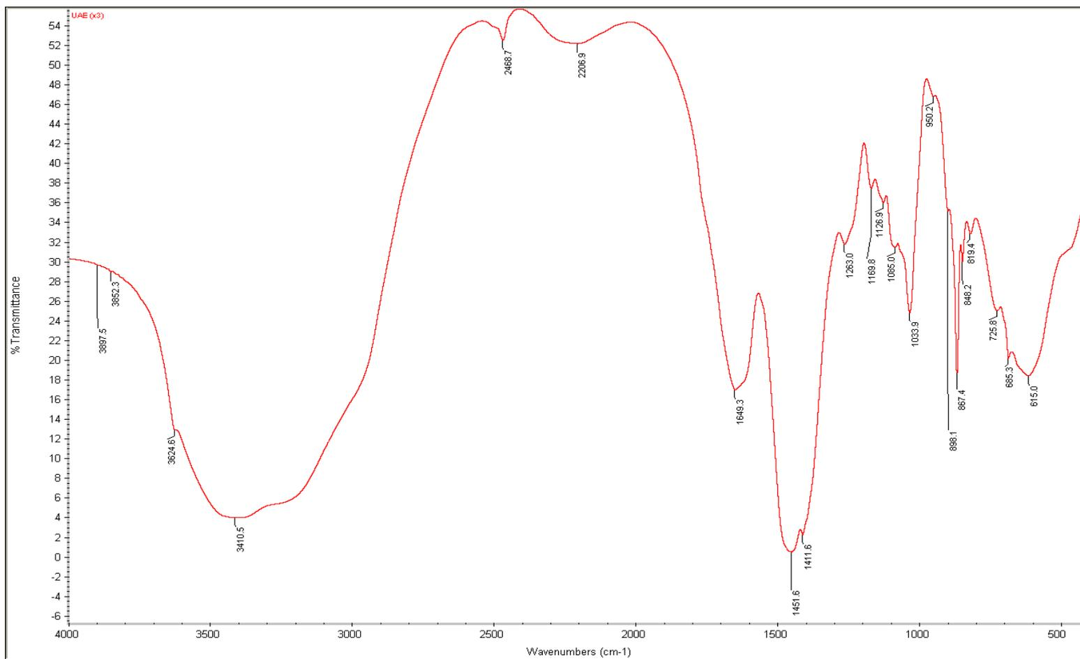
**FIG. B7. THE FT-IR SPECTRUM OF SODIUM ALGINATE EXTRACT FROM ULTRASOUND-ASSISTED EXTRACTION (Alg-UAE) (3×)**
