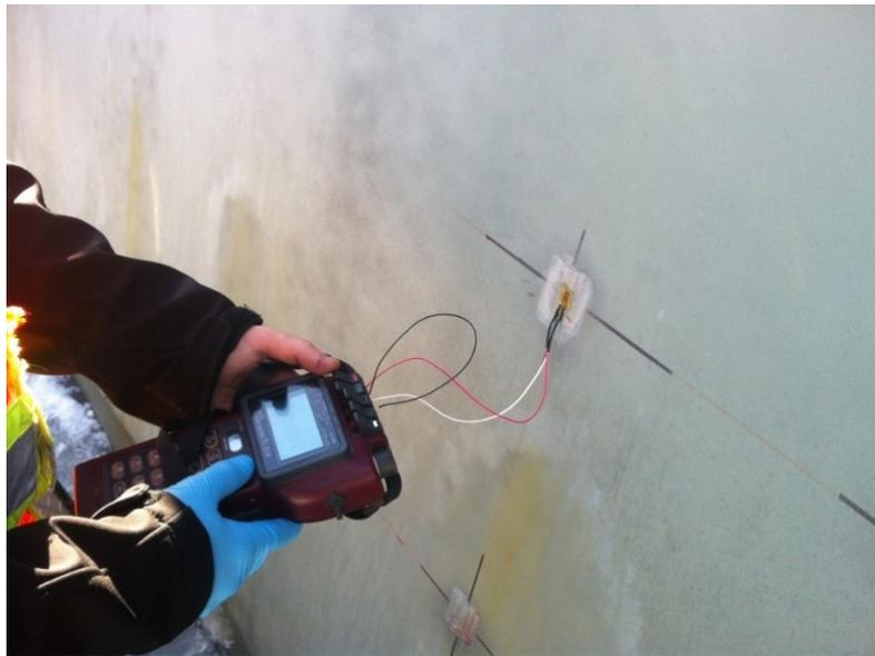
**Figure 3.11: Testing of a uniaxial strain gauge on the inside web of Girder 2**
