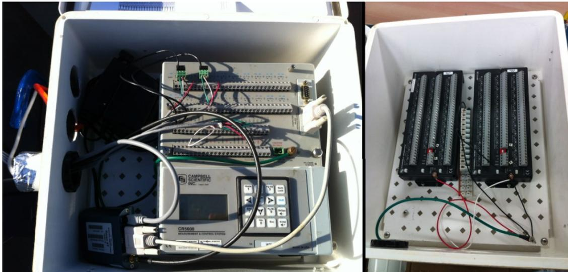
**Figure 3.13: Photos of the CR5000 data logger (left) and two multiplexers (right)**
