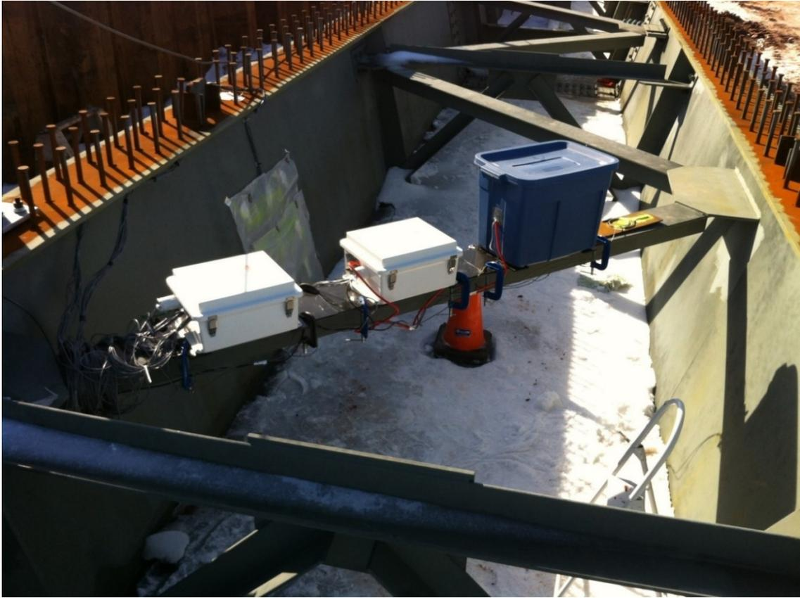
**Figure 3.12: Data acquisition equipment arrangement of Girder 2**
