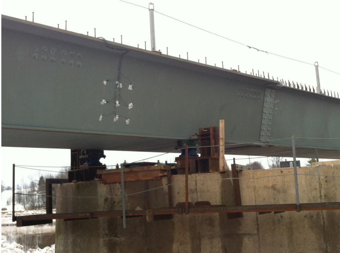
**Figure 3.14: Gauge field of Girder 1 approaching pier 1**
